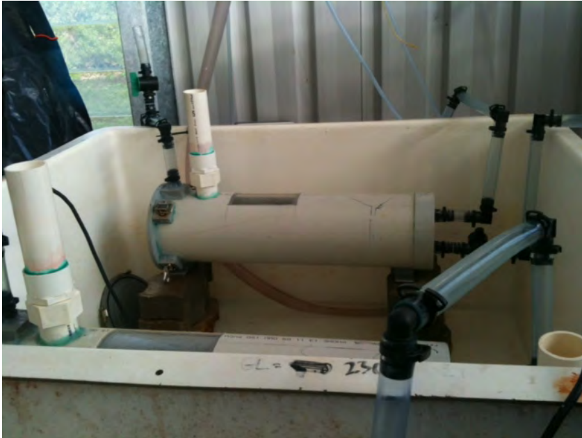
Figure 5. Set-up of respirometer used to measure oxygen consumption of adult S. apama in response to shipping noise.
