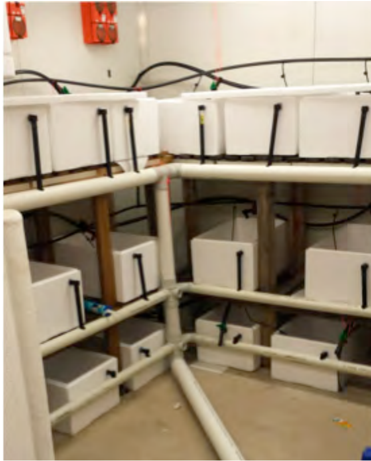
Figure 4. Set-up of flow-through polystyrene holding tanks used to monitor development of S. apama eggs.
